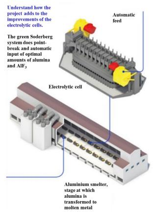
Figure 1. Schematic drawing of the point feeder pots.
